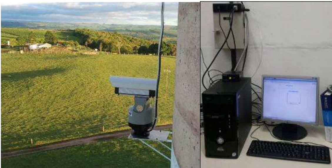
Figure 1. The first LATINELT observation unit. On the left is the camera installed on the top of a pan-tilt unit and fixed on the external wall of the radar building. On the right is the computer, and the hardware box that control the camera and pan-tilt. The whole system is remotely controlled by an operator via internet.
